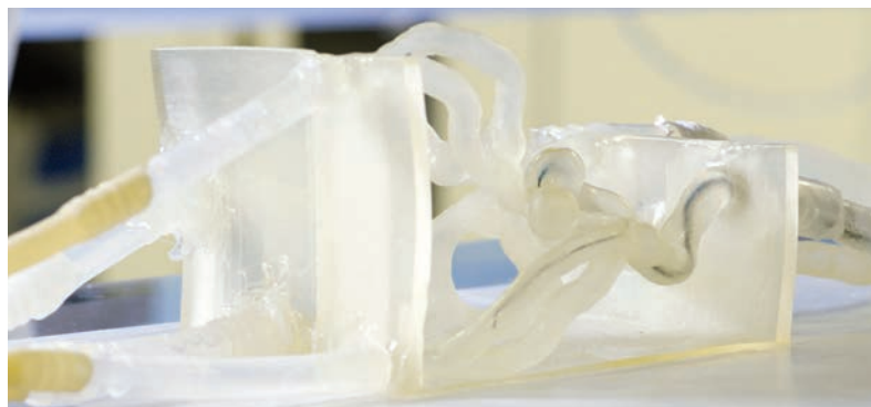
Figure 3. The team at Jacobs Institute tests surgical approaches using a guidewire and 3D printed model which accurately reflects the anatomy of the patient.
