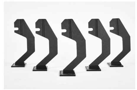
3D printed replacement machinery parts manufactured in under a week using FDM, compared to over a month using traditional methods.
