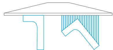
The part on the left is oriented directly against the build head and has a stable center of mass, so it doesn't require supports in this orientation. The part on the right is oriented such that it needs supports.
