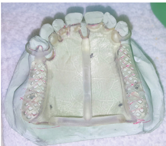
A 3D printed partial framework positioned on a dental model.
