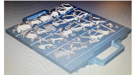
This screen capture of Objet Studio software shows 25 parts loaded on the build tray in preparation for printing.
