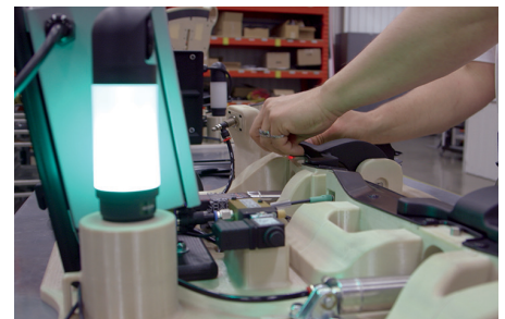
A green light confirms the pins are accurately locked into place and is a validated part.
