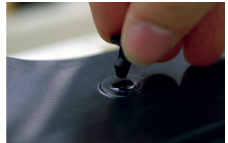
The operator uses pins to lock the part into place.
