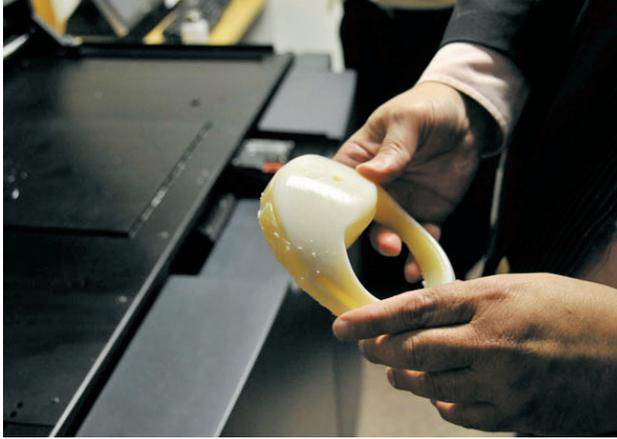
Ivivi's medical device prototype printed on an Objet® 3D Printer.
