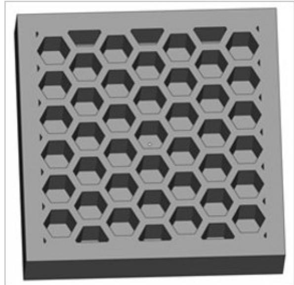
Figure 29: Part using honeycomb exit holes
