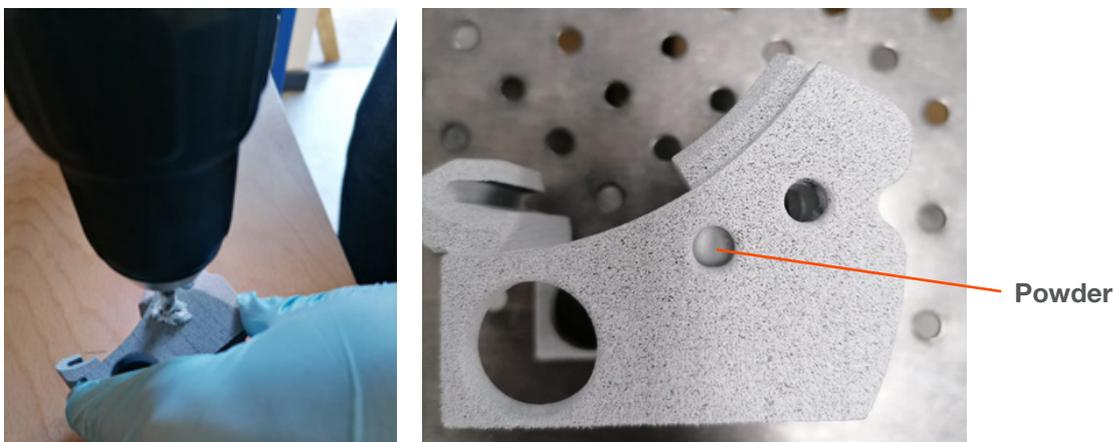
Figure 41: Drilling parts to increase hole diameter and remove powder
