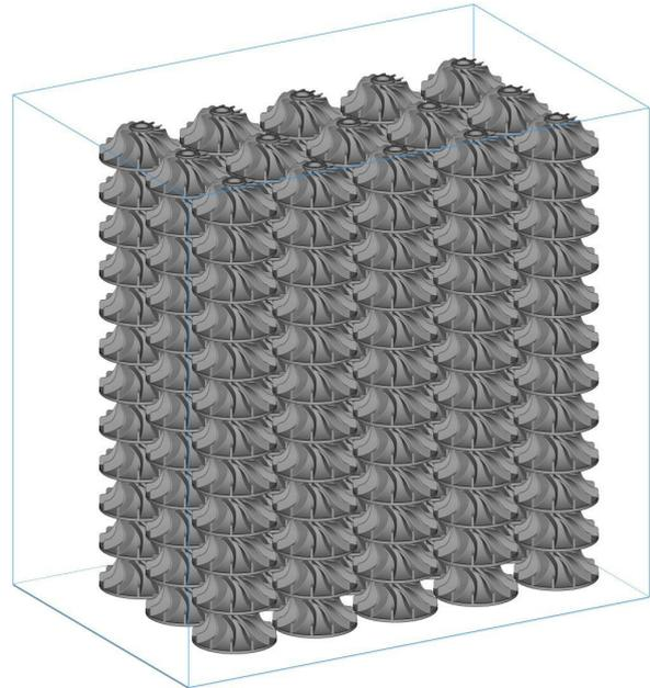
Figure 20: Build density example
